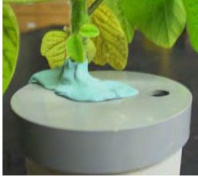
Ensure that the Qubitac is tight around the stem so no gas leaks are formed. Once the gas is being supplied to the pot through the bottom gas inlet, check that gas is coming out of the pot through the gas outlet in the lid. When the T-piece is attached to the gas outlet from the lid and the “PUMP IN” port on the Q-G267, check that excess gas is venting through the T-piece outlet.
