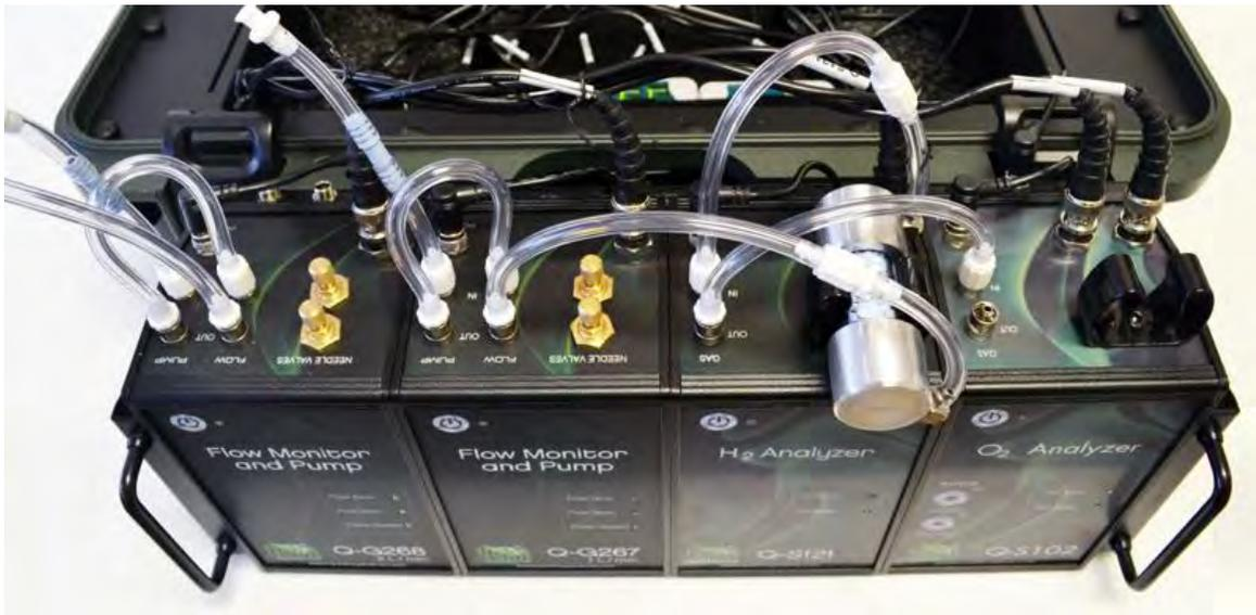
Component Set-Up for Calibration (reference mode)
