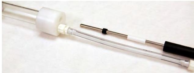
18. Place the nodules in the chamber and attach the chamber to the system in place of the plant pot as shown in item #10 above for an Open-Flow system. Placing the nodules on a moist tissue paper will prevent them from drying out.
