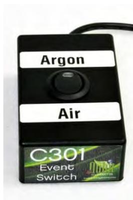
This change in event switch position is necessary for the software to correct the H<sub>2</sub> signal for the background gas used since the output of the H<sub>2</sub> analyzer is affected by the background gas.
