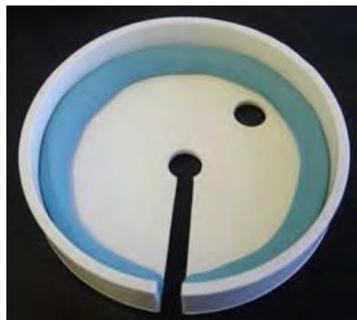
The lid snaps down to seal around the perimeter of the pot while the stem of the plant and the temperature probe are positioned in the slit of the lid. The slit in the lid must then be sealed from the outside with the blue Qubitac sealant to render it gas-tight. Seal the slit by placing a long piece of Qubitac around the plant stem and over the perimeter of the slit and press the Qubitac together and gently down against the lid to seal the plant in the pot.
