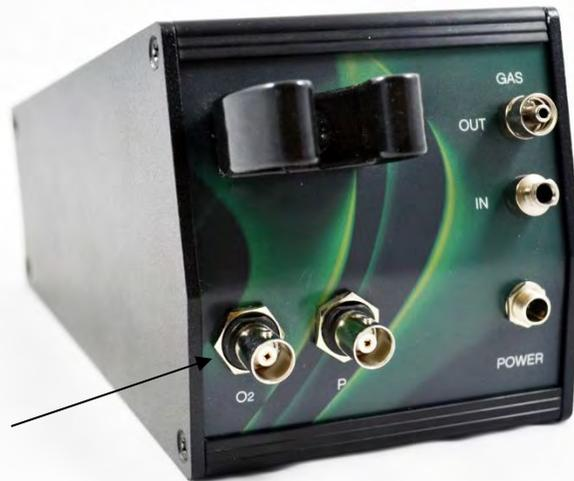
Because of changes in total gas pressure at the O<sub>2</sub> sensor, the O<sub>2</sub> (Pcor) reading in the software (corrected for pressure changes) may not be the same as the Q-S102 O<sub>2</sub> reading. Only at a gas pressure of 100KPa will both the Q-S102 O<sub>2</sub> (kPa) and the O<sub>2</sub> (Pcor) (%) be the same.
