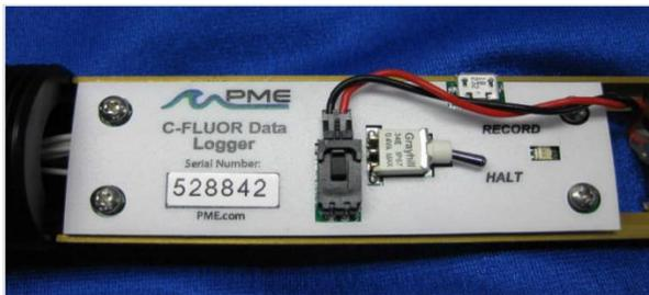
The **LED Light** is an LED that can display either red or green light. This is used to indicate the different features described in Chapter 1 in this manual.
