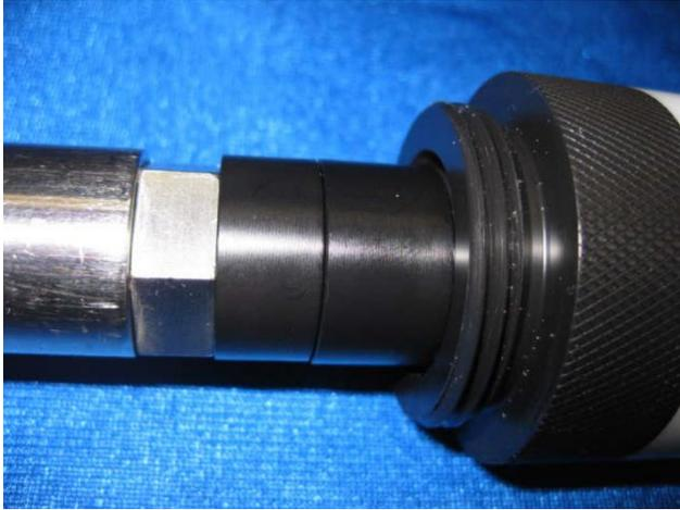
The clip faces will mate. Note that if the clip is not fully screwed onto the connector it will still appear as shown in the picture above, but the sensor may not be making complete reliable contact with the Logger.
