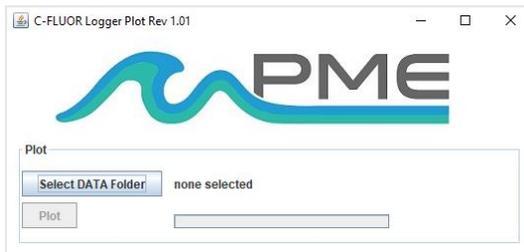
C-FLUOR Plot plots the files recorded by the C-FLUOR Logger. The software reads all Logger files in a folder, except the CAT.txt file.
