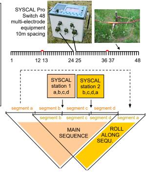
All the SYSCAL Pro Switch units (48, 72, 96, 120) can also be delivered with segments of cables of:
