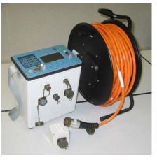
The SYSCAL Pro Switch units use segments (seg) of multi-core cable which are reversible and interchangeable.
