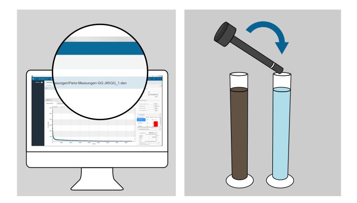
A measurement finishes automatically when the entered duration is over. Alternatively, a user can stop a measurement any time by clicking on the respective button in the PARIO<sup>®</sup> software.
