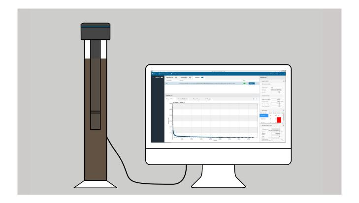
From now on, PARIO Control will record a measurement data triple (time, pressure, temperature) each 10 sec and depicts the recorded data graphically. The status line of the running measurement is moved automatically from the list "In preparation" to the tab "In Progress".
