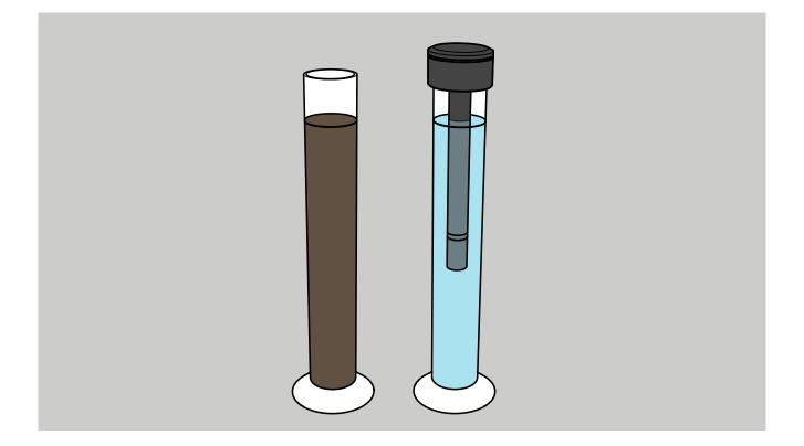
For performing a sedimentation analysis with PARIO<sup>®</sup> you need to place one cylinder with the prepared soil sample and the other one with distilled room tempered water on a plane surface. Insert the PARIO<sup>®</sup> in the distilled water for temperature equilibration and connect it to the computer.
