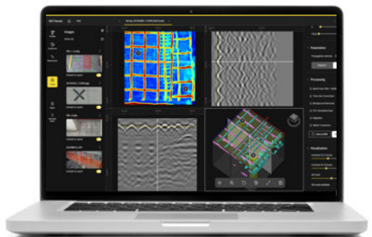
For a comprehensive GPR data analysis, explore different radar views (B-scan, C-scan and 3D model) and survey details (photos, sketches, images).
