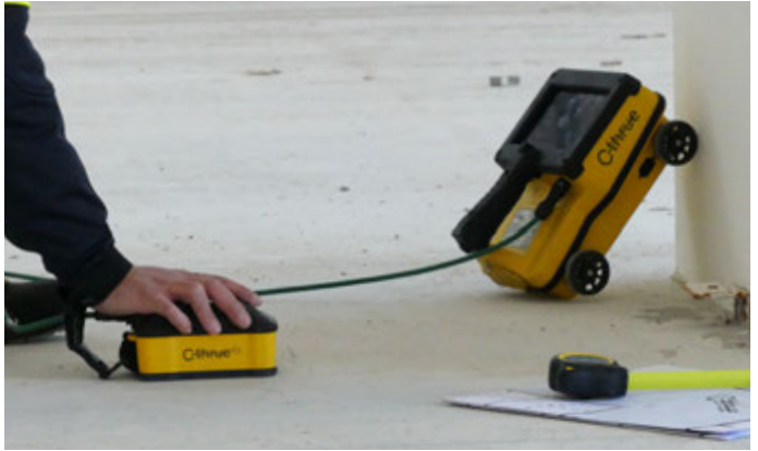
C-thrue XS can be connected via LAN to the C-thrue device allowing for a real-time visualization of the collected data on the multi-touch display.
