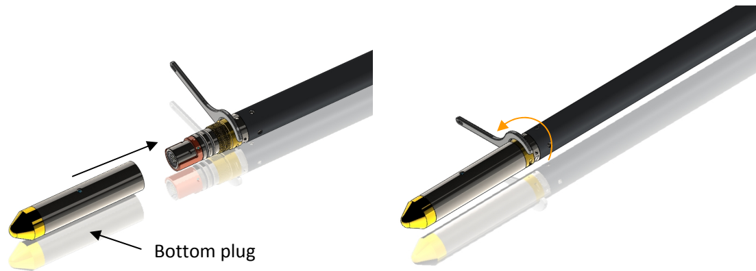
Figure 3-4 Attaching the QL40-Plug
