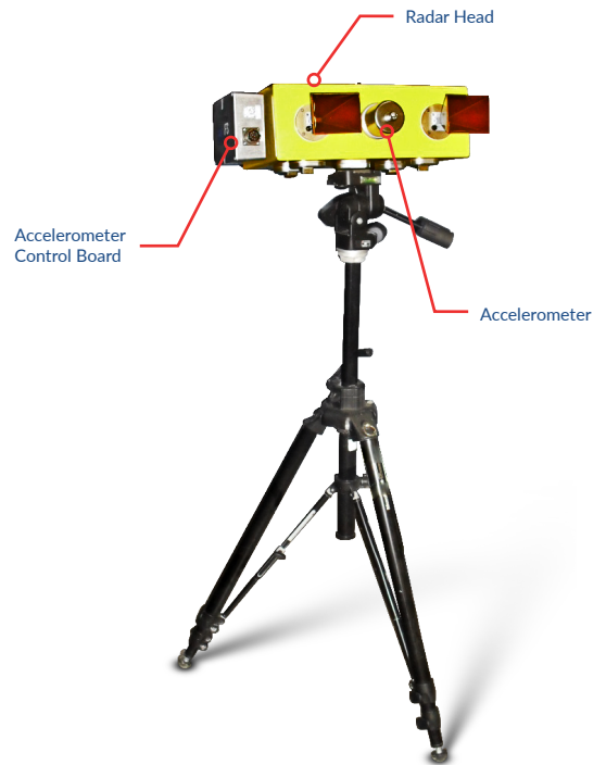
IBIS-FS Plus Incorporates an Accelerometer
