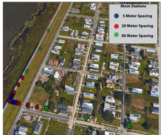
L-shaped array with non-uniform spacing in the Lower 9th Ward, New Orleans, using the Atom Passive Wave Wireless Seismic System.
