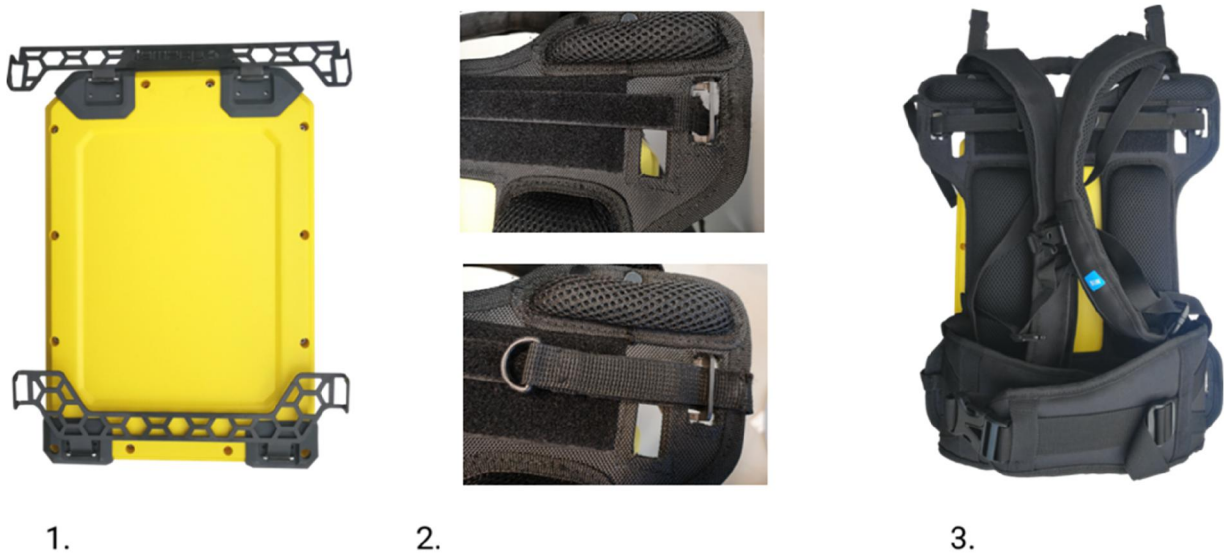
Figure 1. Attaching the backpack harness to GT5000 Terra. 1. Attach the connective metal pieces to the loops on the back of the analyzer. 2. Place the harness on top of the analyzer. Align it so that the loops on the sides of the metal pieces go through the holes on the harness. Pull the Velcro taped strands downwards through the metal pieces, under the edge of the harness, back through the metal loops and attach. 3. Make sure that the harness is well attached.
