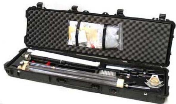
*Fig. 2 Guelph Permeameter Carrying Case.*
