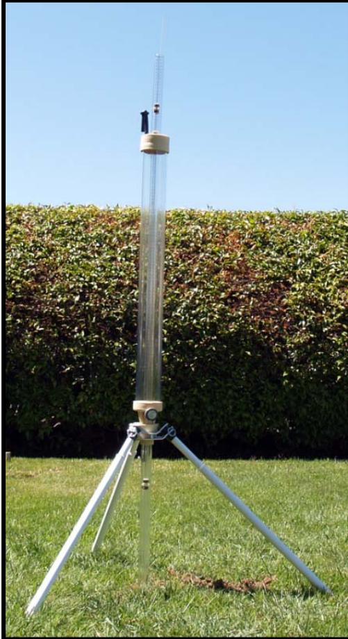
The Guelph Permeameter is an easy to use instrument to quickly and accurately measure in-situ hydraulic conductivity. Accurate evaluation of soil hydraulic conductivity, soil sorptivity, and matrix flux potential can be made in all types of soils. The equipment can be transported, assembled, and operated easily by one person. Measurements can be made in 1/2 to 2 hours, depending on soil type, and require only about 2.5 liters of water.
