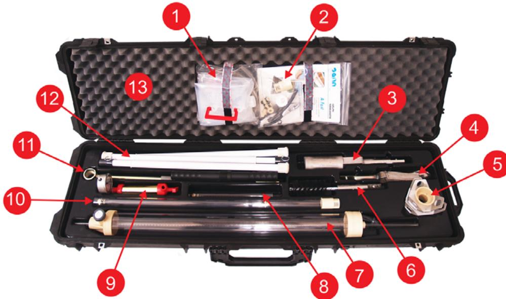
Fig. 5. Guelph Permeameter Kit (2800K1) components in Carrying Case.
